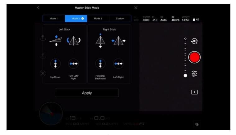
I have my controller set to Mode 2 which means the left stick controls throttle and yaw, and the right stick controls tilt and movement.
