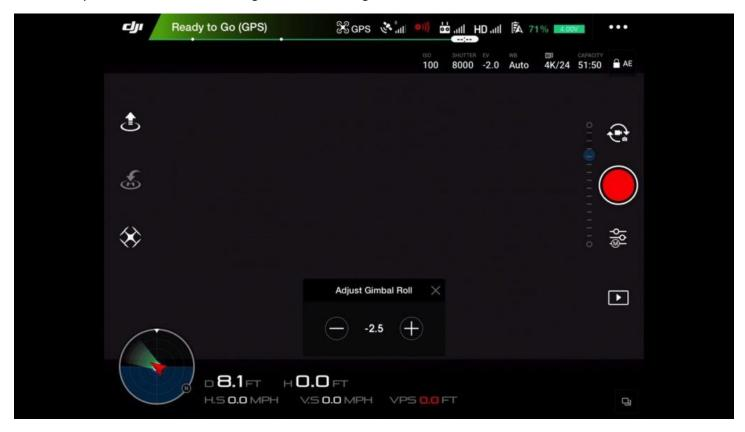
This is handy if you need to temporary fix the orientation of your gimbal if you are out flying since you can fix it remotely without having to bring the drone back for a landing.
