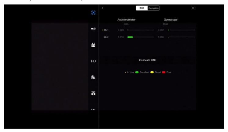
If you have issues with weird flying, drifting or signal and compass errors then try fixing the issue by going through an IMU Calibration.
